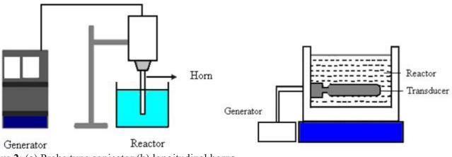
Figure 2: (a) Probe type sonicator (b) longitudinal horns
